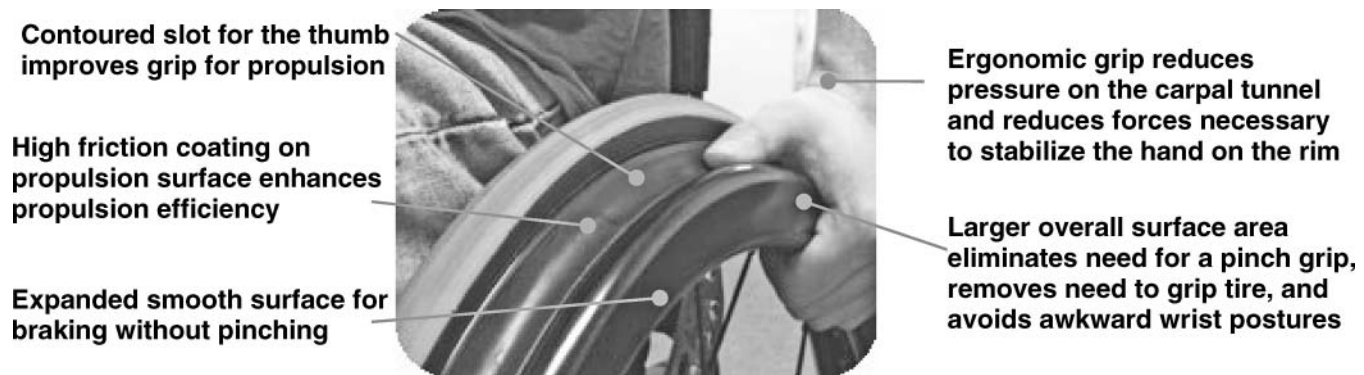
Figure 1. Design features of the Natural-Fit Handrim.
