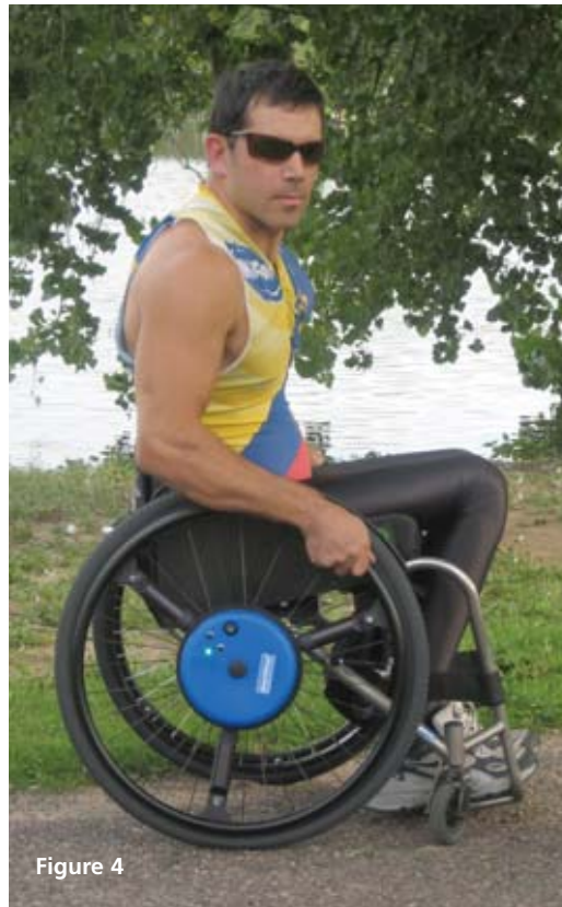
Figure 4. The SmartWheel measurement device mounts to most manual wheelchairs to collect and report propulsion information.
